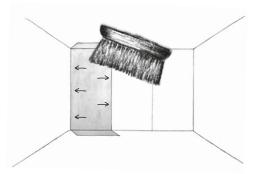
Unroll the panel from the ceilling to the floor. If you are not sure that the ceiling is completely straight, keep 2-3 extra cms of pattern on top.
