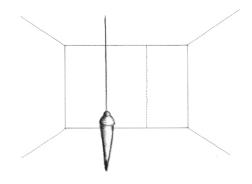
Draw a vertical line from the left corner of the wall, equal to the width of the first panel; use a carpenter's level or a plumb line to help you.
