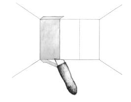
Only <u>after the paste is completely dry</u>, cut what's left of paper on top, bottom & sides. Use a sharp and clean cutter blade, take a new one if necessary.
